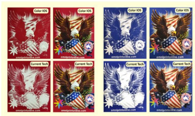
Reduce your white ink usage and the print costs by about 40% with Kotharis Color IOS™. This groundbreaking technology considers the background color of the textile by using it as a print color and adapts the amount of white ink needed for the underbase to print. Depending on the design, the savings can be of up to 70% making this software a must have for the DTG industry.
